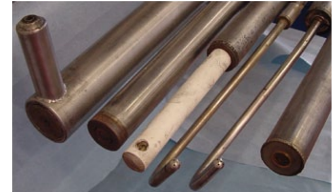
IFRF probes currently available; Three sizes of IFRF external pyrometer shields: the bigger one is used for FOSPER and 500 kW furnace measurements; the middle one is used in the IPFR and the smaller one will be used in TAO.
