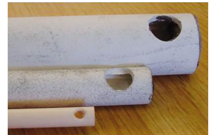
IFRF probes currently available; Three sizes of IFRF external pyrometer shields: the bigger one is used for FOSPER and 500 kW furnace measurements; the middle one is used in the IPFR and the smaller one will be used in TAO.
