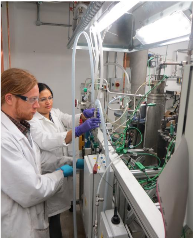
Figure 2: 1\text{kg h}^{-1} continuous bubbling fluidised bed fast pyrolysis reactor.
