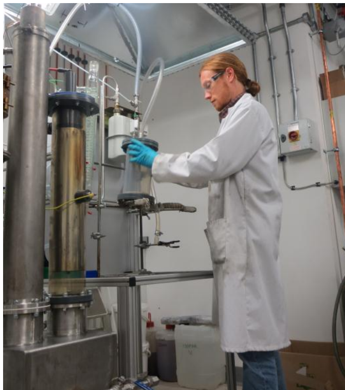
Figure 1: Aston University's 1kg h -1 continuous fast pyrolysis unit.
